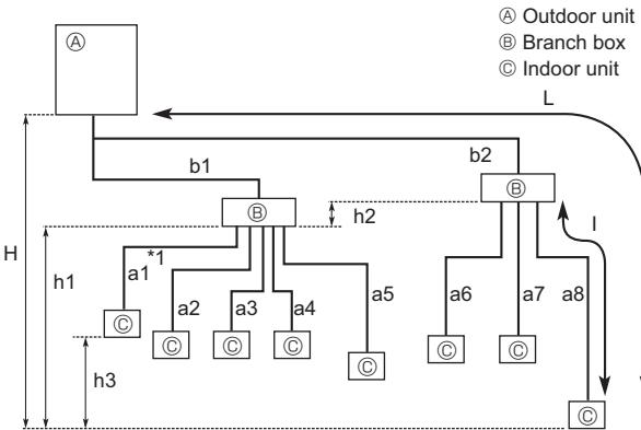
\*1 Although two refrigerant pipes are used between the branch box and the Y-shape connection pipe when connecting the P100 indoor unit, calculate the piping lengths using only the length of one pipe. (Fig. 5-2)
