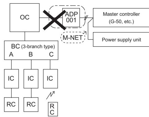
3-1. Plural indoor units cannot be operated by a single remote controller.
