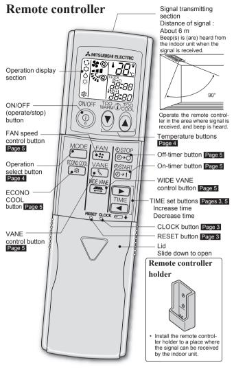
Use the remote controller provided with the unit only. Do not use other remote controllers.
