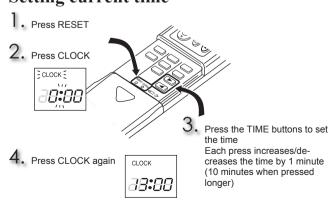
Press RESET and CLOCK gently using a thin stick.
